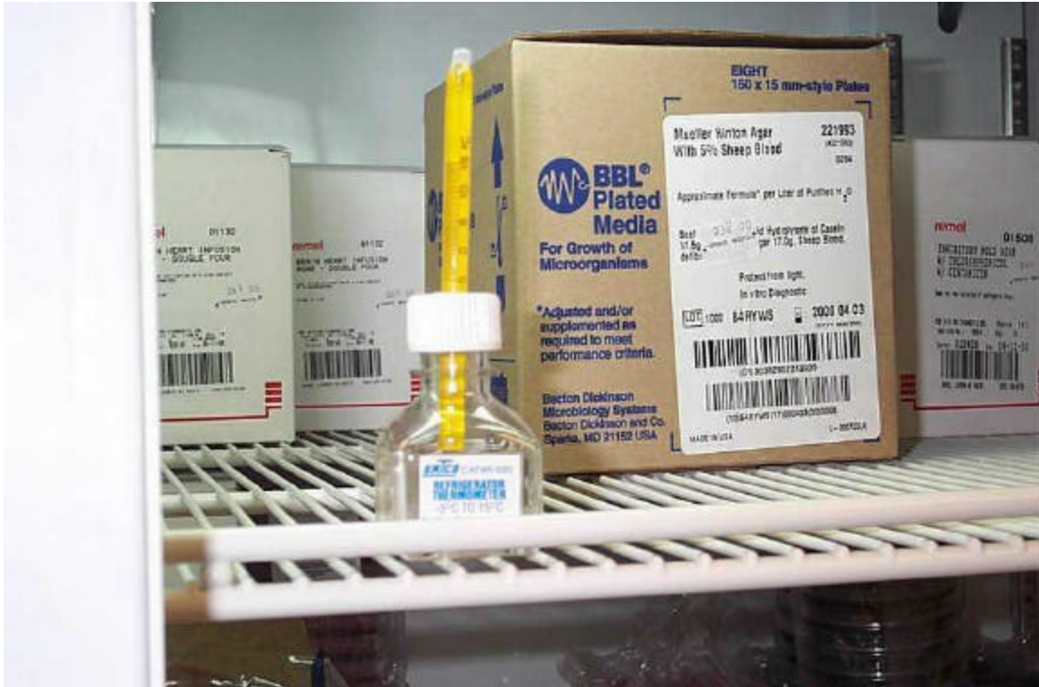
Figure 10 Every hospital refrigerator must have a thermometer. This mercury thermometer could easily be replaced with an alcohol/spirit thermometer. (Pollution Prevention Project Photograph)
