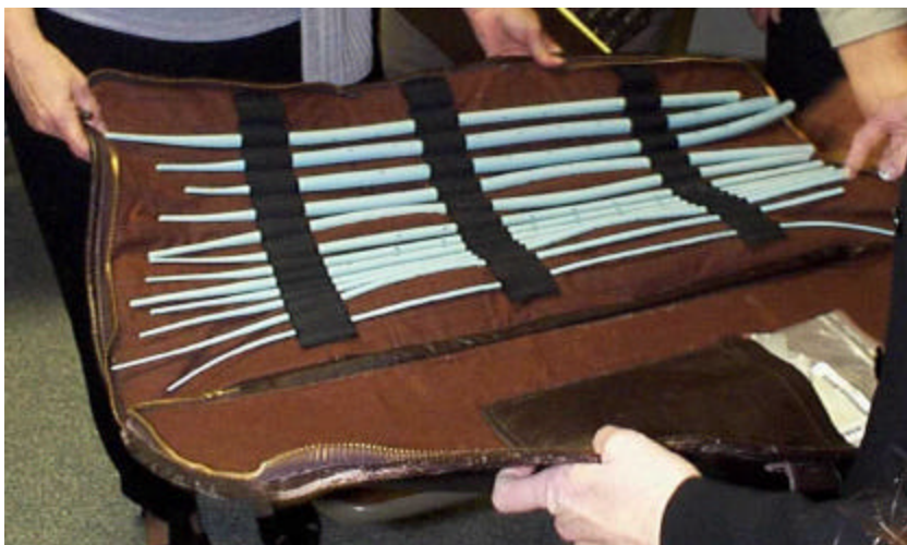
Figure 7 A complete set of tungsten gel-weighted bougies, stored in the leather zippered case that formerly held the mercury ones. (Pollution Prevention Project Photograph)
