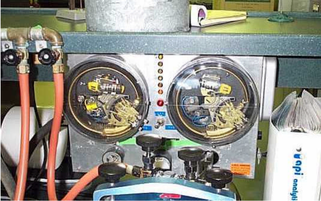
Figure 16 This mercury barostat detects small changes in the vacuum system in the laboratory, switching the vacuum pumps on and off to maintain a constant vacuum. (Pollution Prevention Project Photograph)
