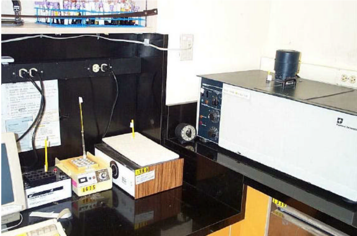
Figure 15 Laboratory thermometers monitor temperatures of various laboratory apparatus, including water bath to the right, heat blocks to the left. (Pollution Prevention Project Photograph)
