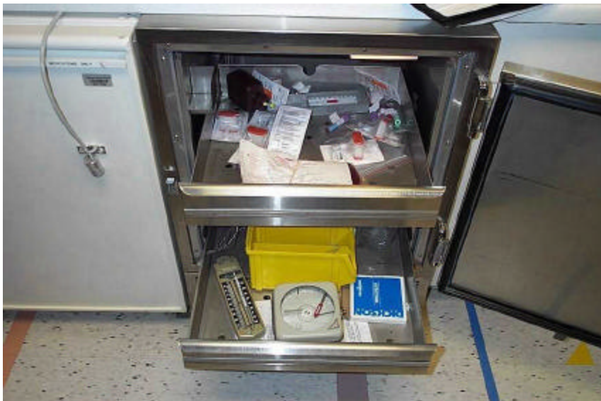
Figure 11 On the bottom shelf of this refrigerator are (left) a mercury minimum/maximum thermometer, and (center) a non-mercury recording thermometer. Uppershelf, at 1 o'clock, a home refrigerator alcohol/spirit thermometer. At 11 o'clock, a "lab quality" mercury one. Mercury thermometers should be replaced with non-mercury thermometers and the number of thermometers in use could be reduced (Pollution Prevention Project Photograph)
