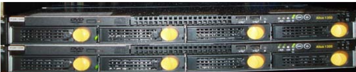
Penguin servers for the WSR-88D. The size of a typical DVD player, this server package is up to ten times more powerful (and ten times cheaper) than the old servers which required an entire 7' x 3' equipment rack..
