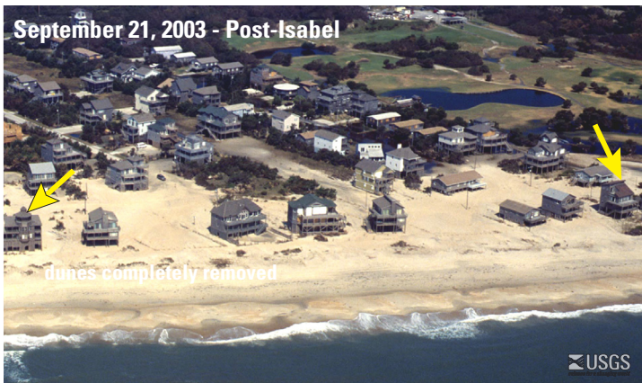
Figure 3. Frisco, North Carolina. USGS aerial photography taken before and after the landfall of Hurricane Isabel. Storm surge and waves overwashed the dunes located seaward of the first row of houses and deposited that sand across the island. (Arrows in all images point to the same features.)
