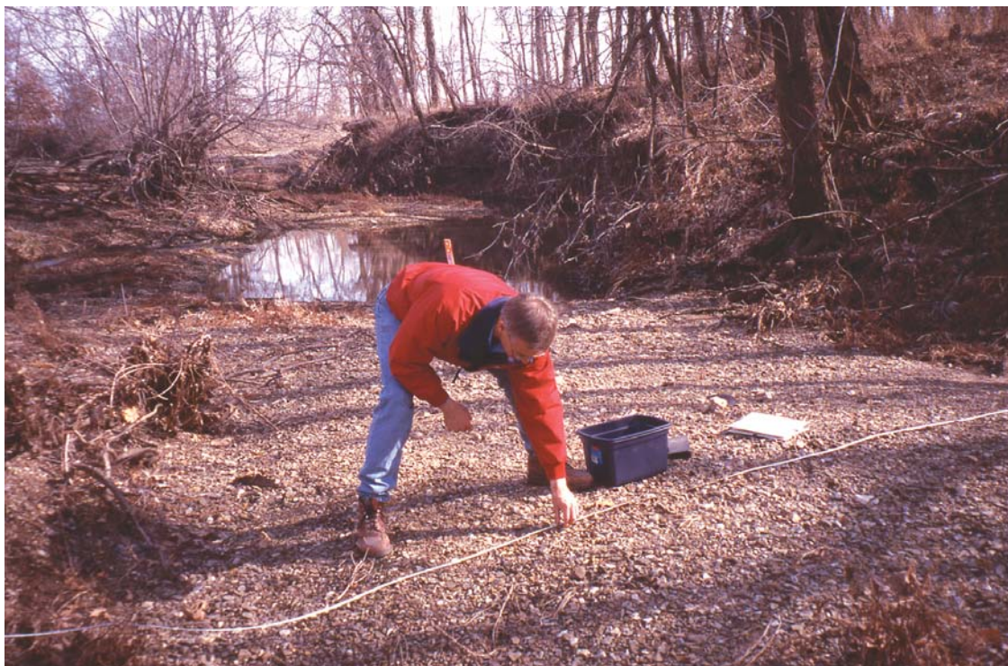
Figure 5. Collection of a random sample of gravel for subsequent particle-size analysis. Location is Indian Creek site 1 (fig. 1B). Photograph taken on February 27, 2004.
