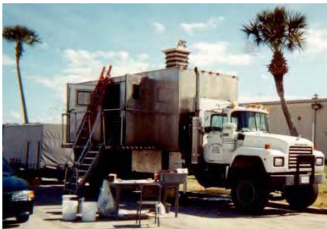
Figure 4-4. Outdoor Cone Penetrometer Test Rig for Soil Coring at Launch Complex 34
