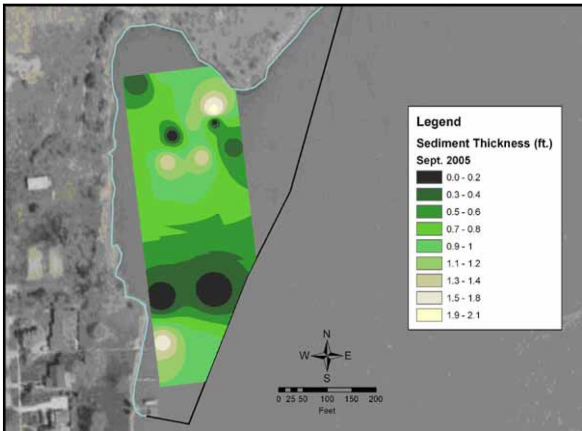
Figure 6-2 Black Lagoon Sediment Thickness After Completion of Phase II Dredging (based on data collected in August and September 2005)
