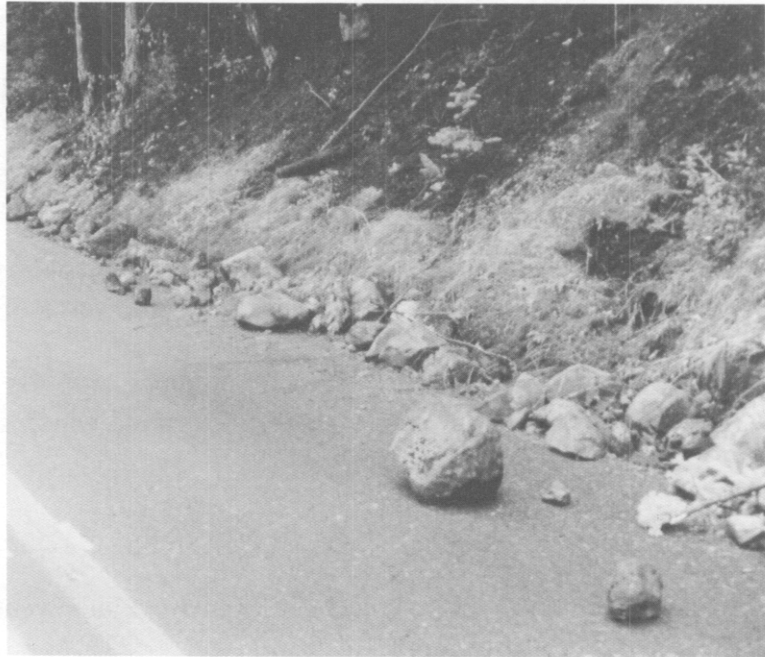
Figure 5.28 Block size used to rate this event.
