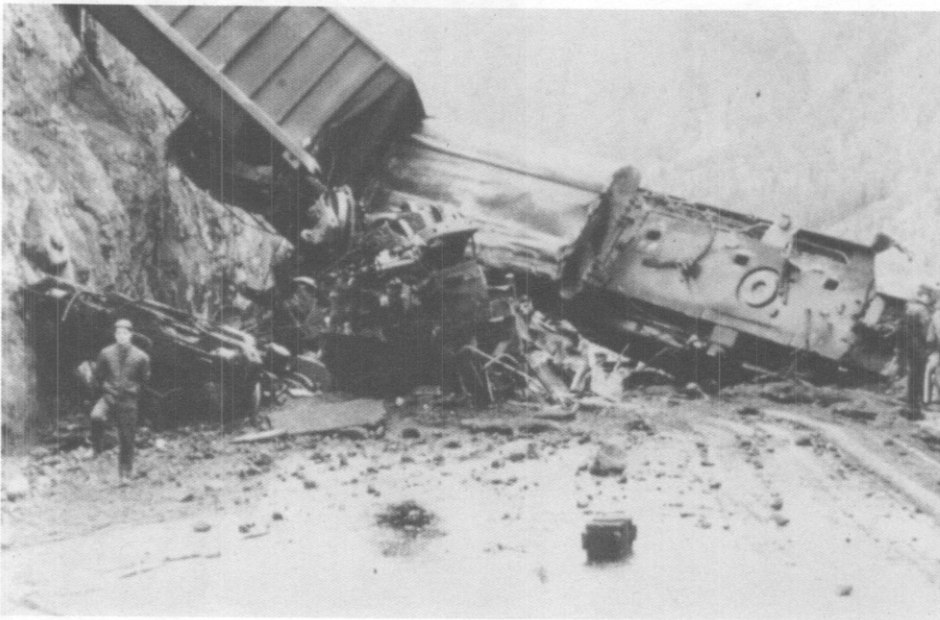
Figure 1.2 Railroad accident caused by a rockfall.
