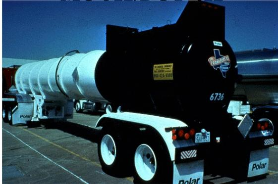
General requirements applicable to all DOT specification cargo tanks are contained in 49 CFR 178.320. General design and construction requirements applicable to Dot 400 series tanks may be found in 178.345. The specifications for a DOT-407 cargo tank may be found in 49 CFR 178.348.
