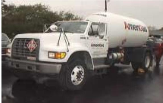
General requirements applicable to all DOT specification cargo tanks are contained in 49 CFR 178.320. The specifications for a MC-331 cargo tank may be found in 49 CFR 178.337.
