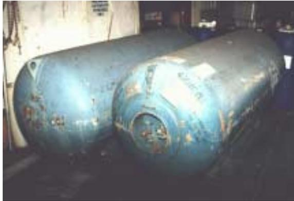
**The specifications for a DOT 57 portable tank may be found in 49 CFR 178.245. The specifications for a DOT 60 portable tank may be found in 49 CFR 178.255.**
