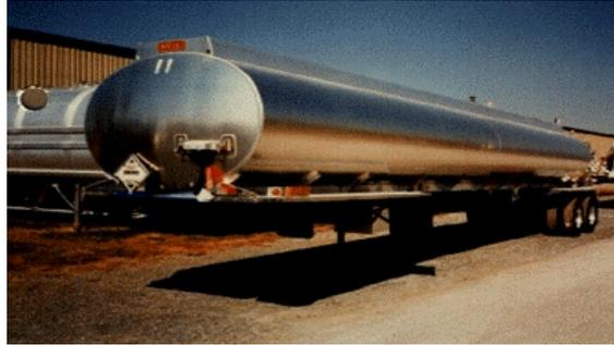
**General requirements applicable to all DOT specification cargo tanks are contained in 49 CFR 178.320. General design and construction requirements applicable to Dot 400 series tanks may be found in 178.345. The specifications for a DOT-406 cargo tank may be found in 49 CFR 178.346**
