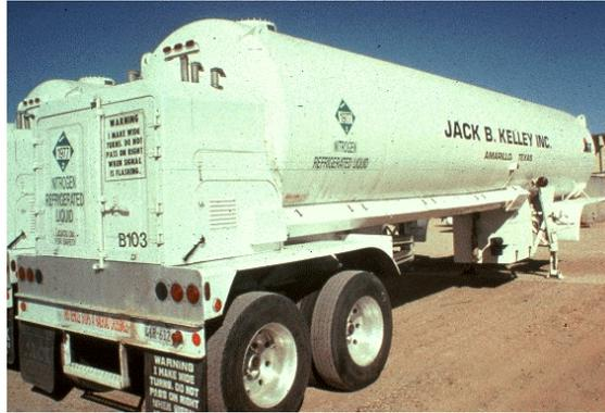
General requirements applicable to all DOT specification cargo tanks are contained in 49 CFR 178.320. The specifications for a MC-338 cargo tank may be found in 49 CFR 178.338.
