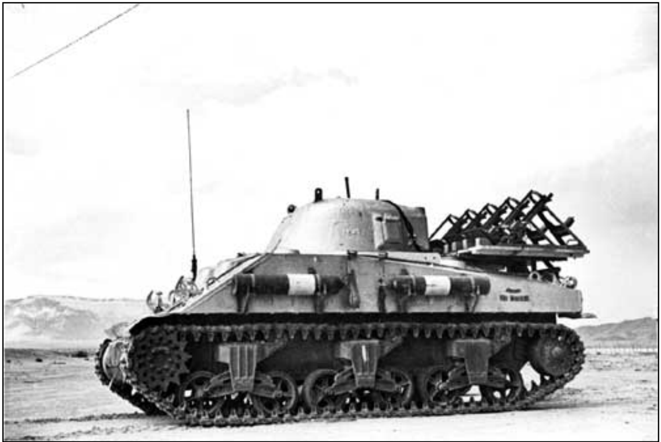
Figure 42. Special "Sherman" tank out-fitted for soil sampe collection (1945). ( Courtesy Los Alamos Photographic Laboratory )
