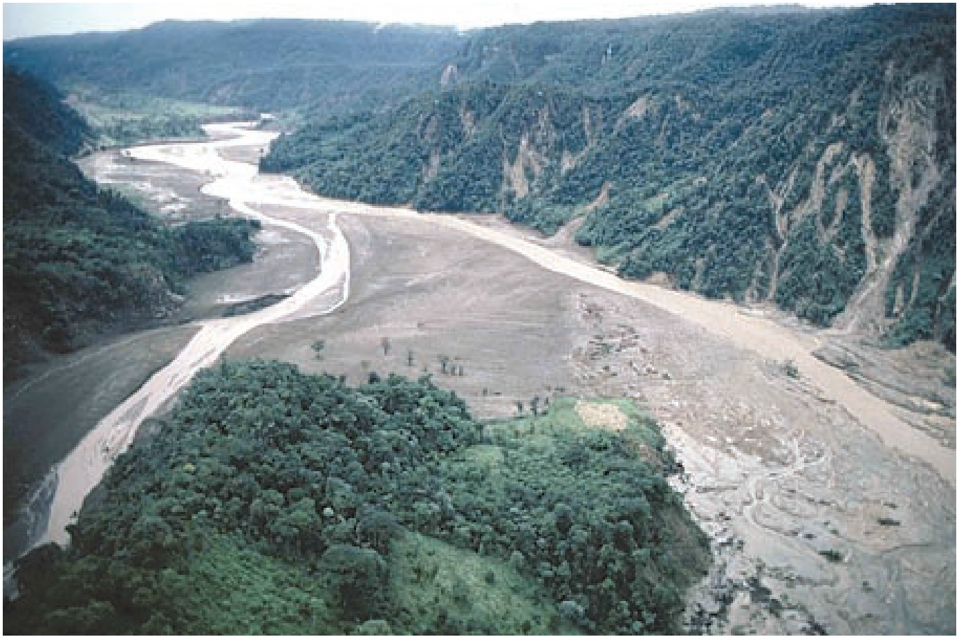
Figure 31. View looking downstream at the confluence of the Río Malo (flowing from lower left) and the Río Coca, northeastern Ecuador, in South America. Both river channels have been filled with sediment left behind by debris flows triggered by the 1987 Reventador earthquakes. Slopes in the area had been saturated by heavy rains in recent days before the earthquake. Debris/earth slides, debris avalanches, debris/mudflows, and resulting floods destroyed about 40 kilometers of the Trans-Ecuadorian oil pipeline and the only highway from Quito. (Photograph by R.L. Schuster, U.S. Geological Survey; information from Reference 32.)
