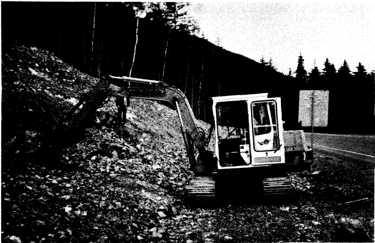
Figure A-80.—Trenching with a backhoe at the Road Cut gold-copper prospect. This prospect was discovered by Bureau personnel at a location 3 miles south of Haines during 1986 (J. Still, photographer).
