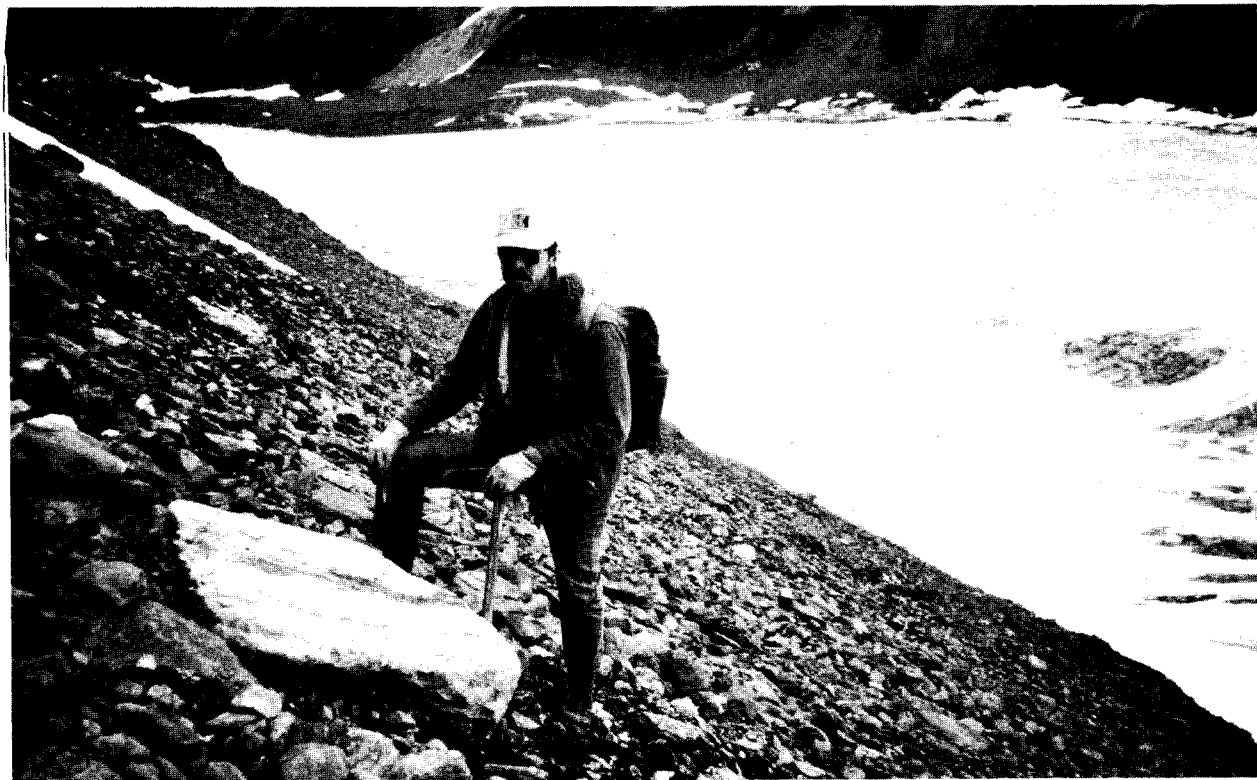
Figure A-18.—Bureau of Mines and ADGGS personnel examine a 6-ft thick sphalerite boulder in gully number 4 of the Mount Henry Clay prospect. A chip sample across this boulder assayed 33% zinc. Such massive sulfide boulders found along a glacier terminus for a distance of 3/4 mile led private companies to diamond drill through the glacier and narrow rock ribs in the hopes of discovering the bedrock source of the boulders. Below, a 2-foot thick sphalerite-barite boulder located between gully number 3 and 4 (J. Still, photographer).
