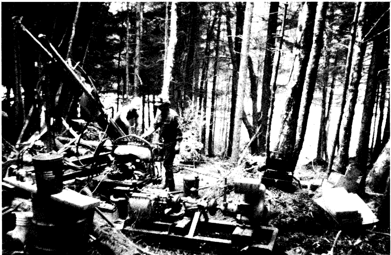
Figure A-81.—Diamond drilling the Road Cut prospect during 1987. Above, drilling off a flat bed truck to intercept the down dip extension of the Road Cut mineralization at a depth of 20 feet below the surface. Below, this hole is inclined at 45° and was drilled to intercept the down dip extension of the Road Cut mineralized zone at a depth of 120 ft below the surface (J. Still, photographer).
