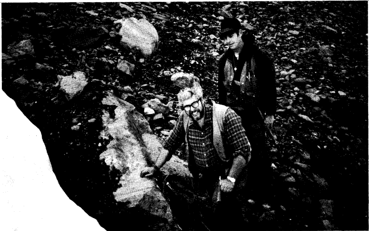
Figure A-18.—Bureau of Mines and ADGGS personnel examine a 6-ft thick sphalerite boulder in gully number 4 of the Mount Henry Clay prospect. A chip sample across this boulder assayed 33% zinc. Such massive sulfide boulders found along a glacier terminus for a distance of 3/4 mile led private companies to diamond drill through the glacier and narrow rock ribs in the hopes of discovering the bedrock source of the boulders. Below, a 2-foot thick sphalerite-barite boulder located between gully number 3 and 4 (J. Still, photographer).
