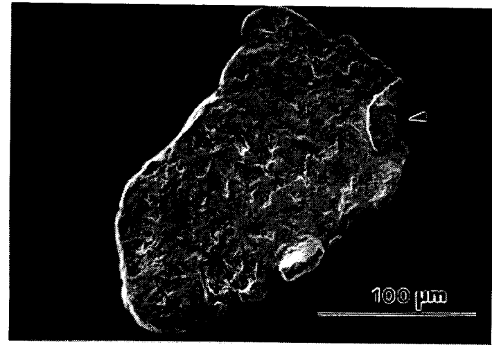
Figure 24f. -- Typical flattened gold grain from Cape Yakataga beach sands. Note folded edges on grain.
