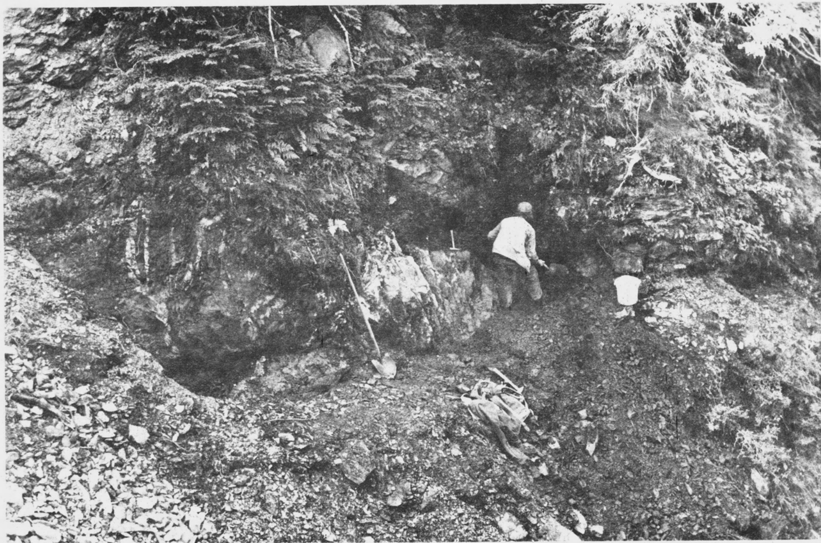
Figure 49. - The 1585 foot elevation pit dug on the Falcon Arm Prospect to locate the source of gold-rich quartz float. Samples taken across a narrow quartz vein that runs from below the rock hammer to the middle of the shovel assays from 0.49 to 1.70 oz. gold per ton.
