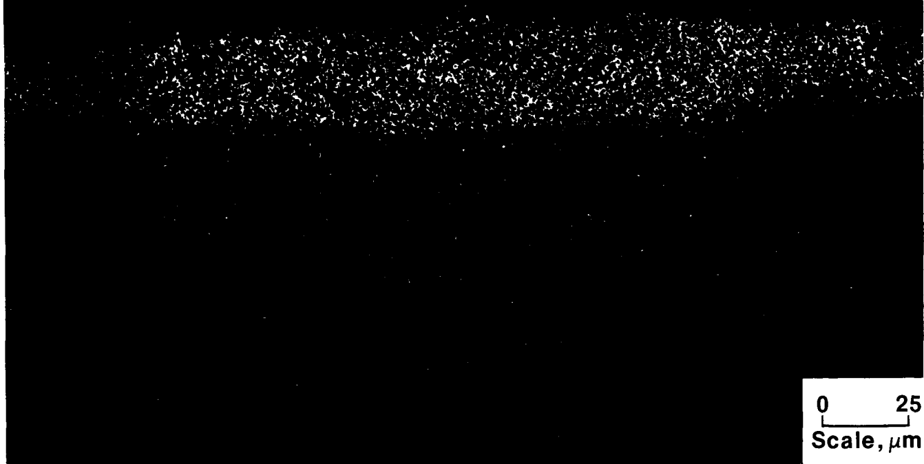
FIGURE 2.—Energy-dispersive X-ray map showing Cr in the cross section of Fe-5Cr substrate with an initial 3-mm-Cr coating after laser processing. Alloyed region is 25 to 30 mm thick with an average composition equivalent to Fe-15Cr.
