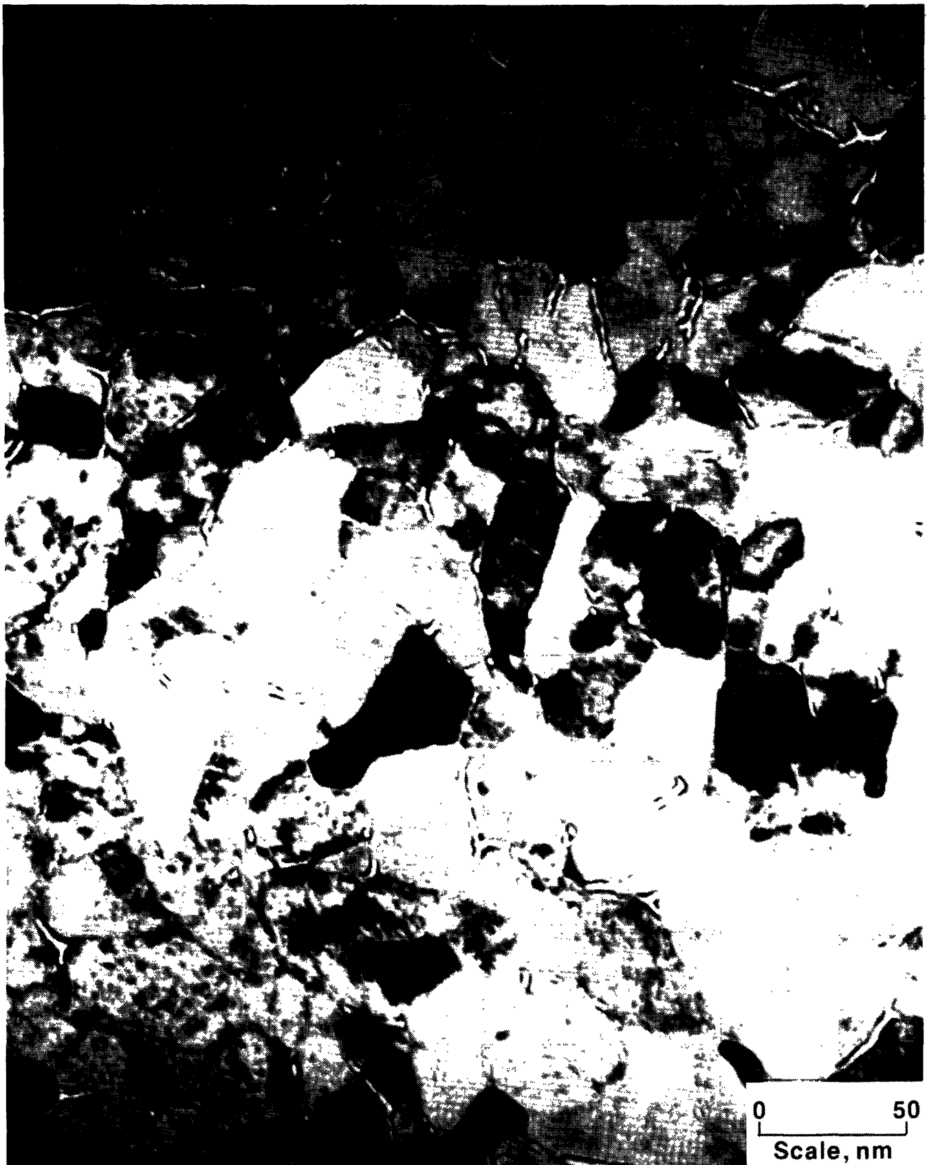
FIGURE 4.—Bright-field transmission electron micrograph of a vapor-quenched (at 77 K) 304 stainless steel film exhibiting intergranular voids and small grains. Picture is overfocused to show voids (29).
