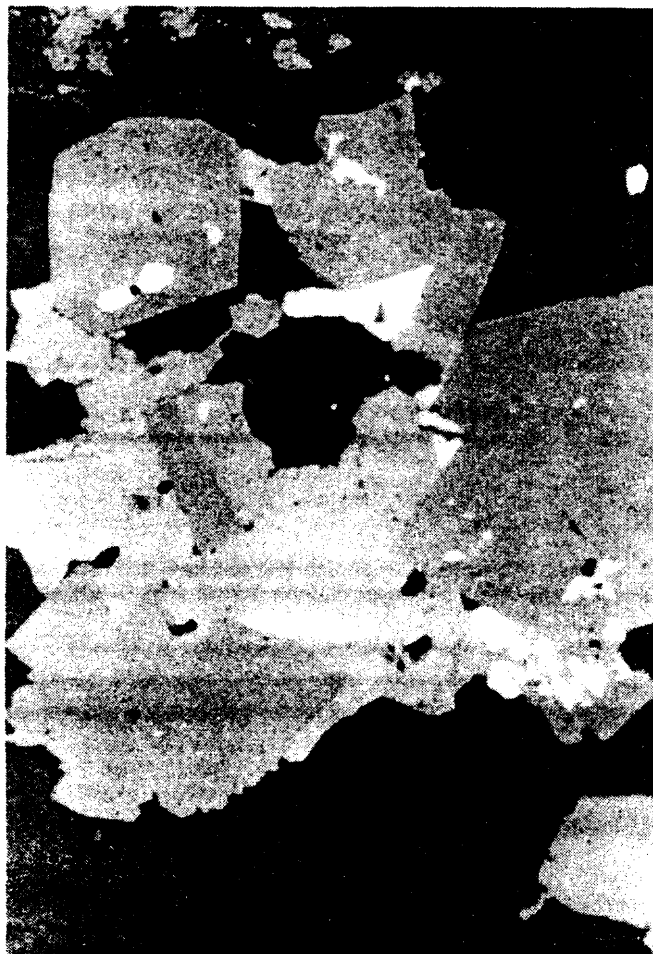
Figure 4.—SEM backscatter electron photomicrograph of multiphase grain with pyrite (gray), galena (white), and sphalerite (light gray) (X 500).
