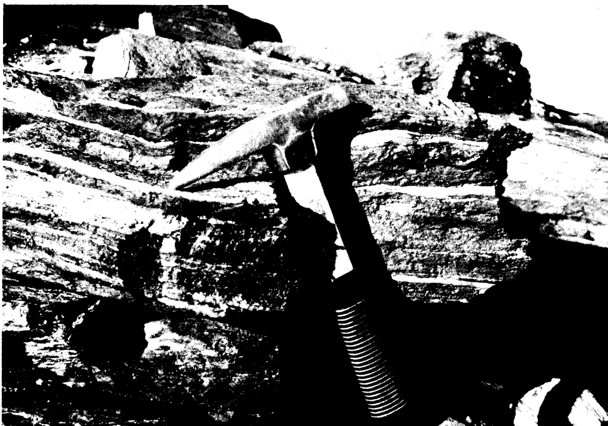
Figure C-5.—Stratiform arsenopyrite-pyrite mineralization at the Dream Prospect. Three Bureau samples across 2-6 inch sections of these layers averaged 55.5 ppm gold and 5.6% arsenic.
