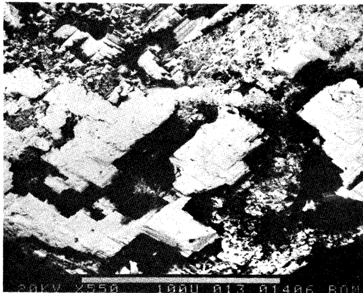
FIGURE 23-B. - Enlargement of lower center portion of sperrylite grain in above photograph. The platy crystalline growths (?) are composed of isoferroplatinum. Note scale bar is 100 microns.
