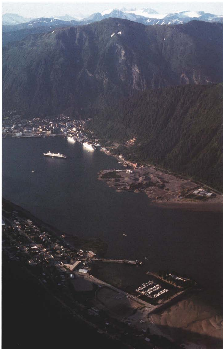
The cities of Juneau and Douglas. At the middle right of the photo are the waste-rock and tailings dump from the Alaska Juneau Mine and the remains of the mill. At the bottom right of the photo are the tailings from the Treadwell mine 300- and 240-stamp mills (Juneau Gold Belt subarea).
