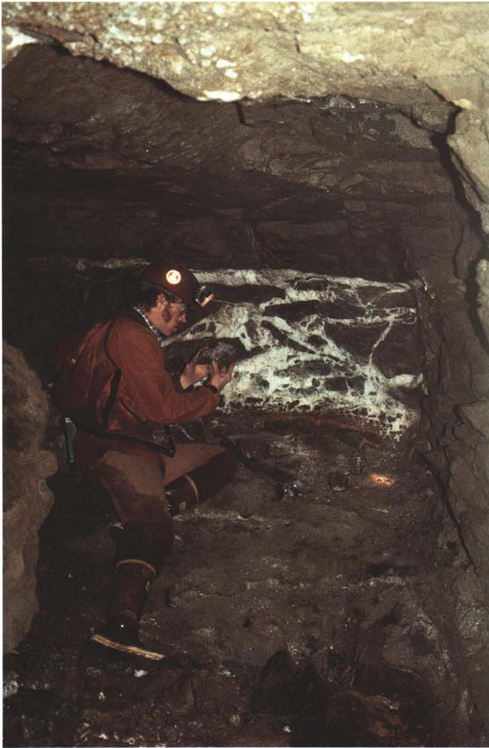
Examining quartz-filled breccia in a thrust fault at the Crystal Mine (Juneau Gold Belt subarea).
