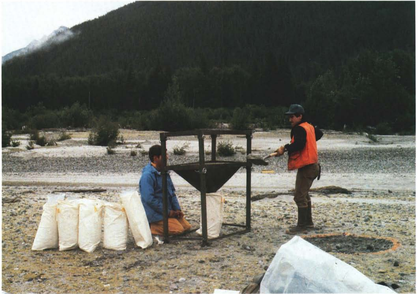
Bureau personnel sample sand and gravel resources at Lace River as part of the industrial minerals portion of the Juneau Mining District study.
