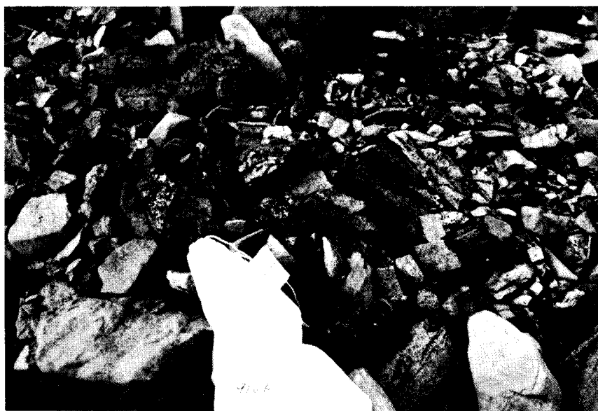
Figure 25. - Photograph of disseminated, coalescent, and massive chromite bands in dunite rubblecrop at Siniktanneyak Mountain.
