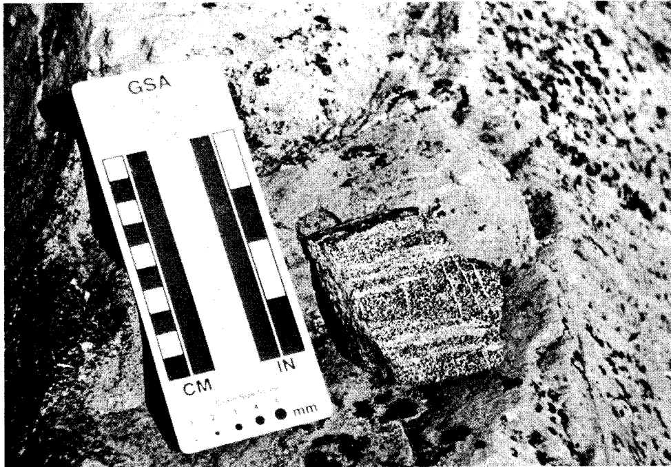
Figure 6. - Photograph of banded coalescent chromite in dunite in the Avan Hills.
