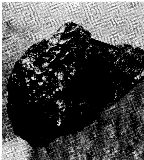
Figure 10. - Osmiridium grain recovered from argillite talus at Miller Gulch (map number 88). Grain is 3 millimeters along longest axis.
