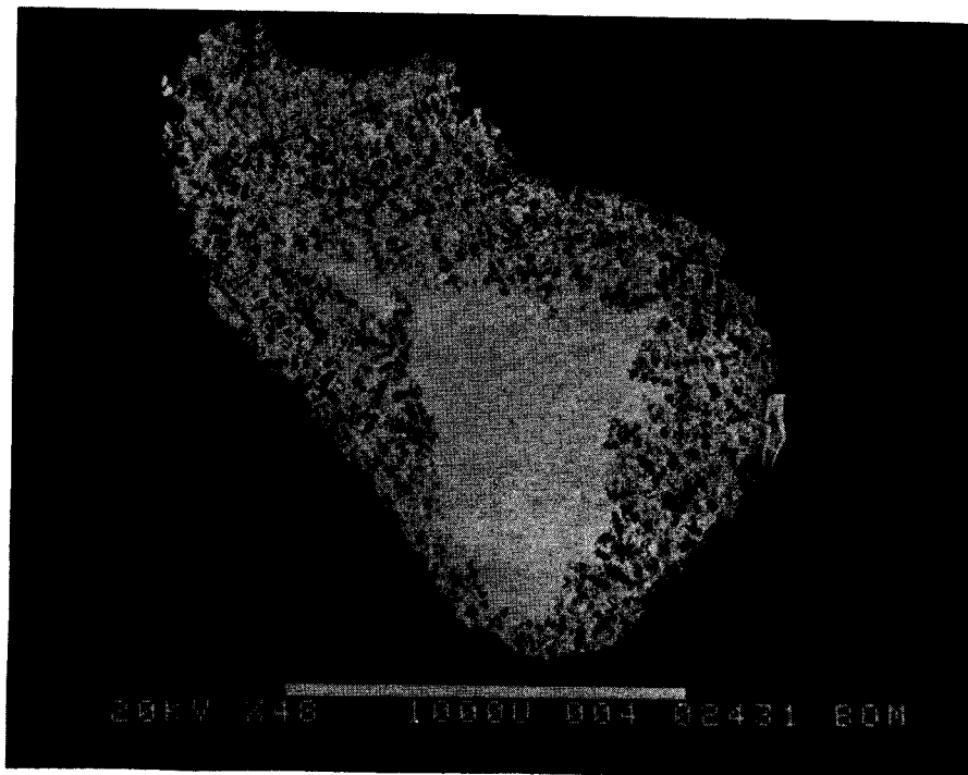
Figure 13. - Back-scatter SEM image of dendritic native gold in native lead placer grain from Miller Gulch. Traces of silver, antimony, sulfur, and arsenic were also detected during energy-dispersive X-ray analysis. Scale bar is 1,000 microns (1 millimeter).
