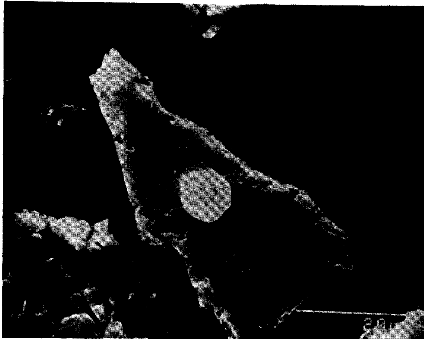
Figure 16.- Back-scatter SEM image of equant 7-micron gold particle in quartz fragment from crushed argillite sample from Miller Gulch. Scale bar is 20 microns (0.02 millimeters).
