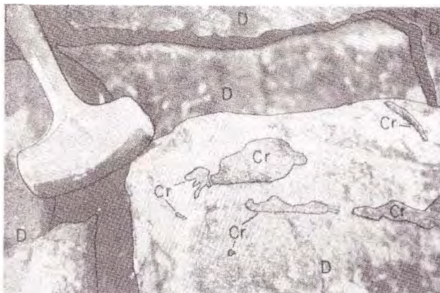
FIGURE 9. - Chromite pods in dunite.
