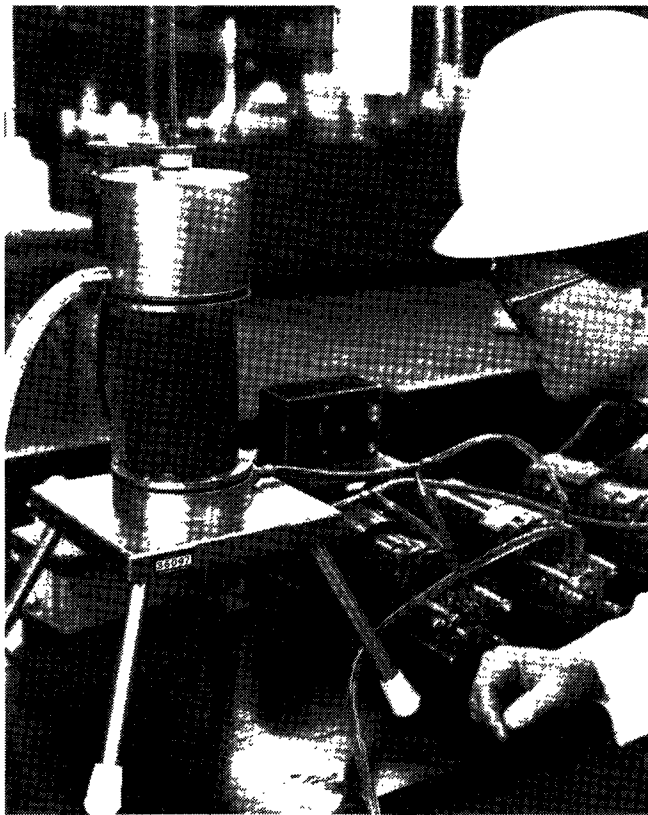
Figure 6.—High-rate thickener sizing test unit.
