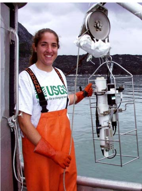
Deploying the CTD instrument in Glacier Bay.
