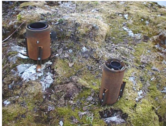
Figure 2. Typical monitoring set up at climate sites. Upper left photo shows white solar radiation shield housing temperature sensors and a tipping bucket rain gauge installed on 1-meter tall post at the McBride Glacier site. Photo on lower right shows the tipping bucket and electronic rain gauges in steel housings as mounted on the ground at the Sun Dew site. A post is only used where animals are unlikely to damage rain gauges, but preferred to reduce snow cover effects early in the winter season.
