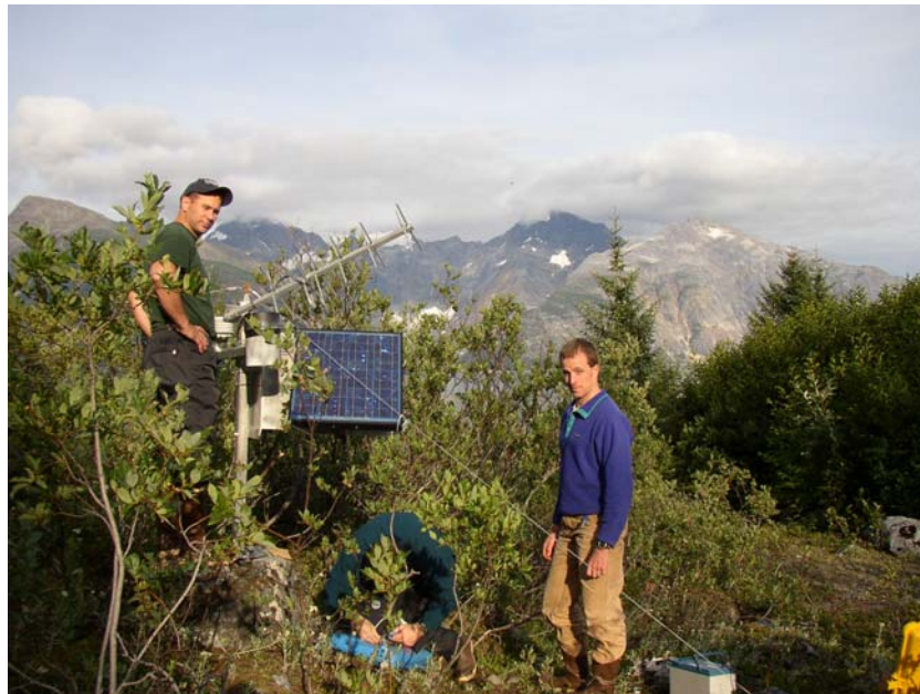
Figure 3. GOES test site in Queen Inlet. GOES satellite transmission system transmits hourly data on precipitation and air temperature, while also storing these data as a backup on Campbell data logger located within the grey box.
