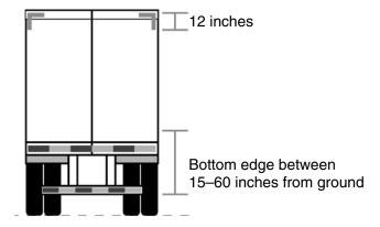
For flat-bed trailers, the rear tape must be has shown:
