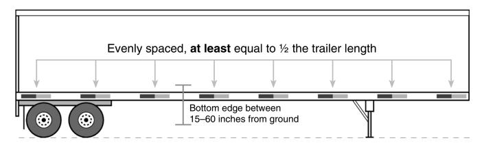
For box trailers, the rear reflective tape must be as shown:
