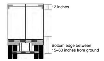
For flat-bed trailers, the rear tape must be has shown:
