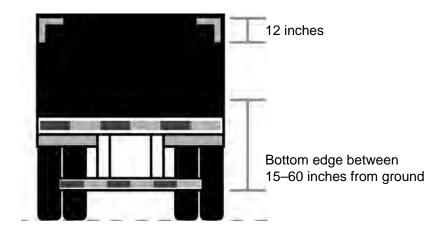
For tanker trailers, the rear tape must be has shown:
