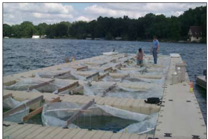
Figure 3. Floating dock holding the large (2-m wide \times 11-m deep) plastic cylinders called mesocosms. Each of these mesocosms may be thought of as a miniature lake.
