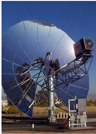
Remote Dish-Stirling system technology is used to capture solar energy
