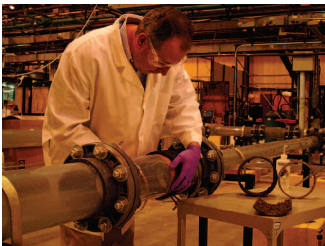
An EPA scientist prepares to test real-time, online sensors for water distribution systems. The sensors detect changes in water quality that would result from the intentional release of chemical and biological contaminants.
