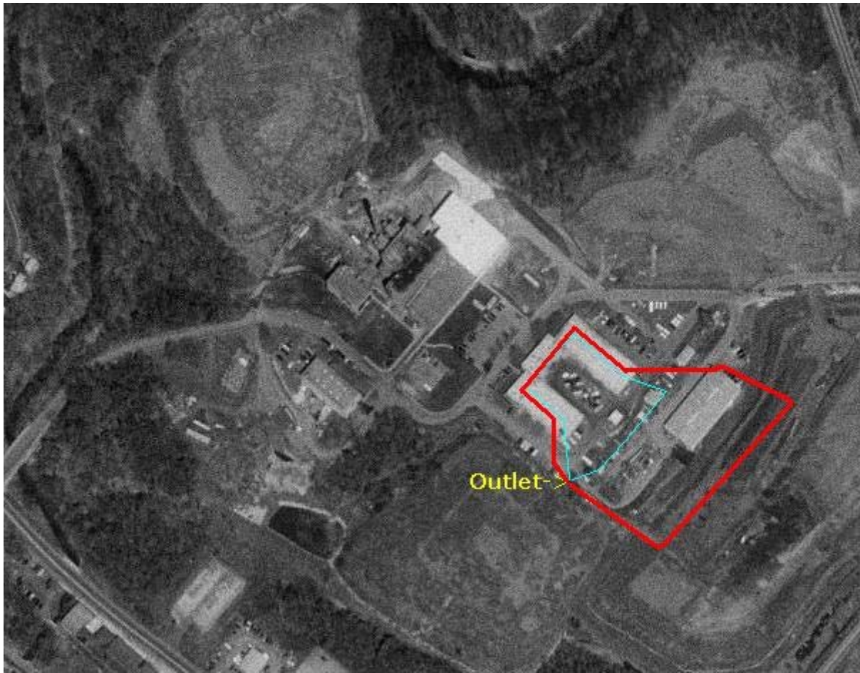
Figure 3-2. Aerial photograph of Harrisburg Public Works Yard showing outlet and drainage area delineation.
