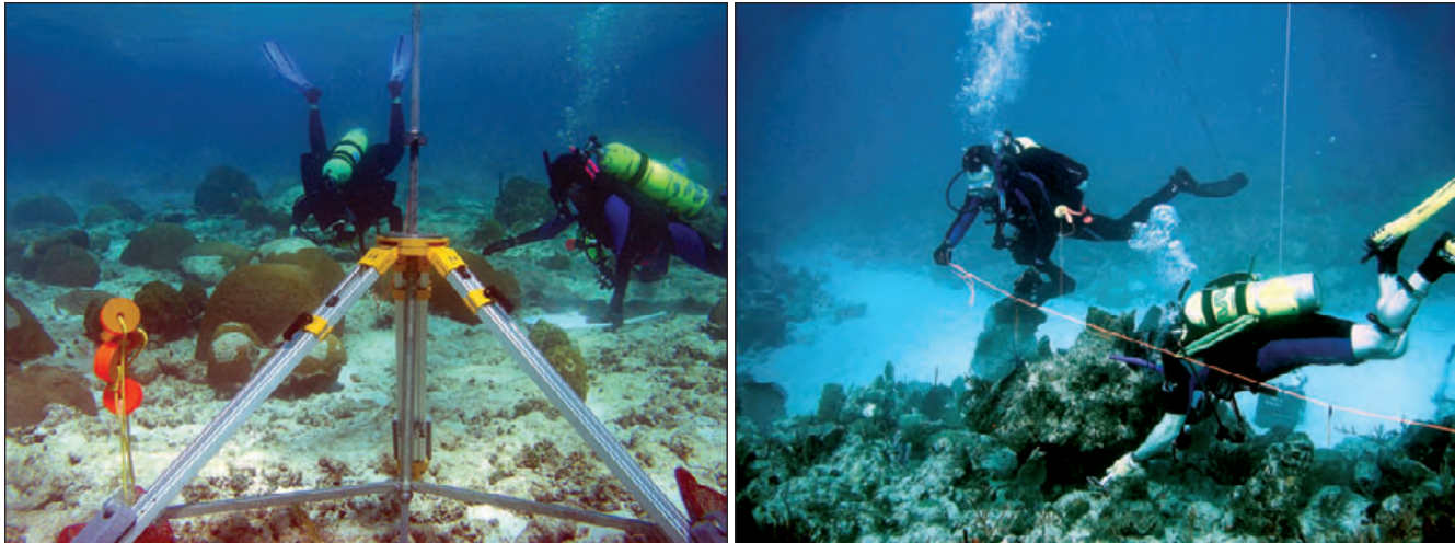
Figure 3-5. A radial-belt transect is established with a fixed stake (permanent station) or temporary tripod (left) at its center. A line is extended from the center and held above the colonies by the line tender (right). Weighted flags or beads are suspended from the line to mark the 2-m width of the belt transect).
