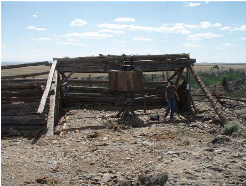
Lander Field Office – Carrie Shields Mine project, showing Karina Bryan, LFO archaeologist, just to the right of the horse whim that was reconstructed. The post sticking out from the whim is what the horse would have been attached to.
