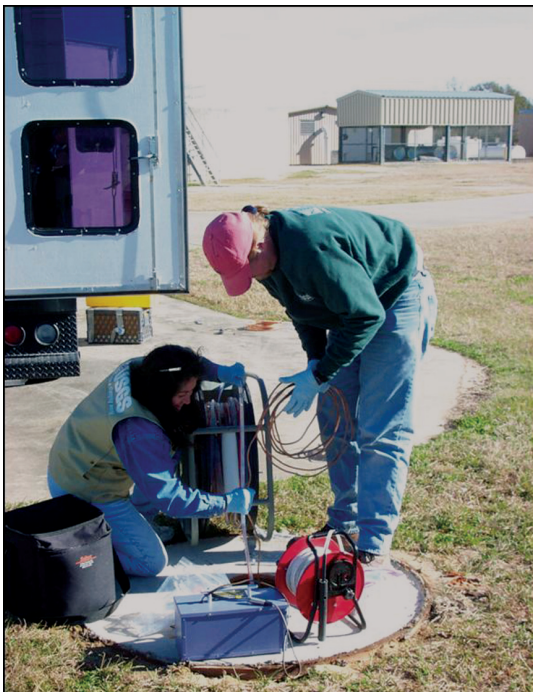
USGS personnel sample a shallow monitoring well in an urban area. Nitrate concentrations measured by NAWQA from 1992 to 1999 at nearly 2,000 shallow wells were used to develop the nitrate model.
