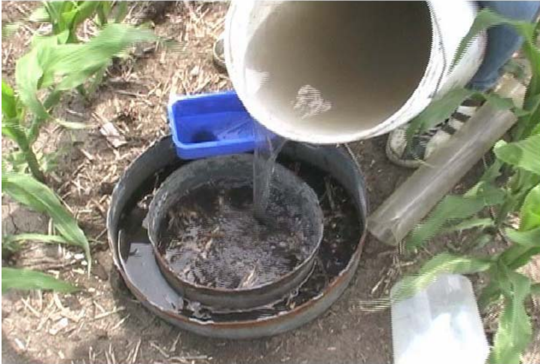
Figure 2. Double ring infiltrometer to measure infiltration rates after manure application.
