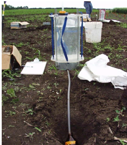
Figure 3. Microsprinkler system used to examine infiltration and antibiotic runoff from soil after manure application.
