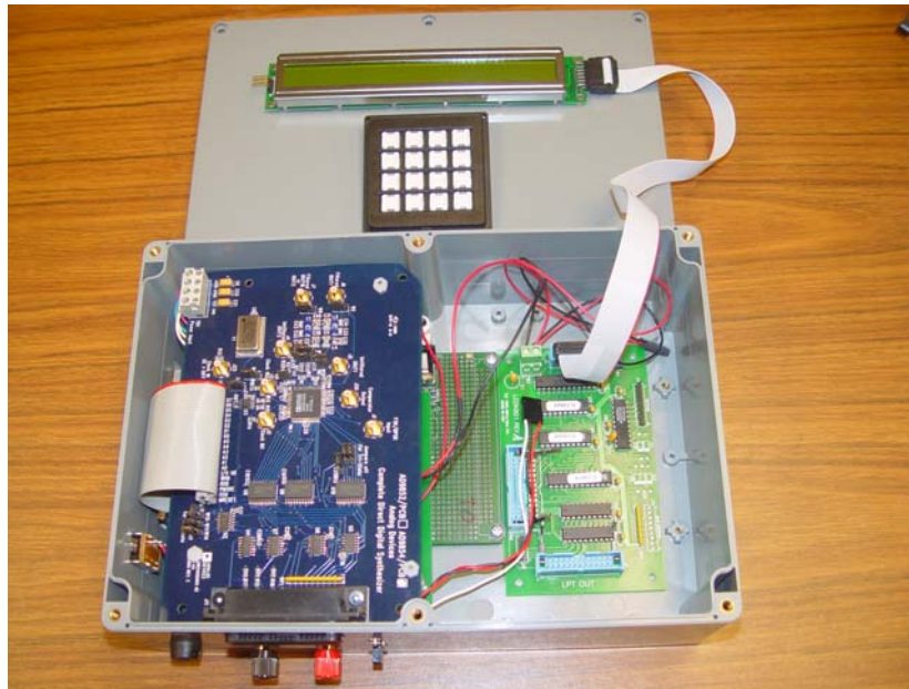
Figure 3. Signal conditioning/processing and user interface
