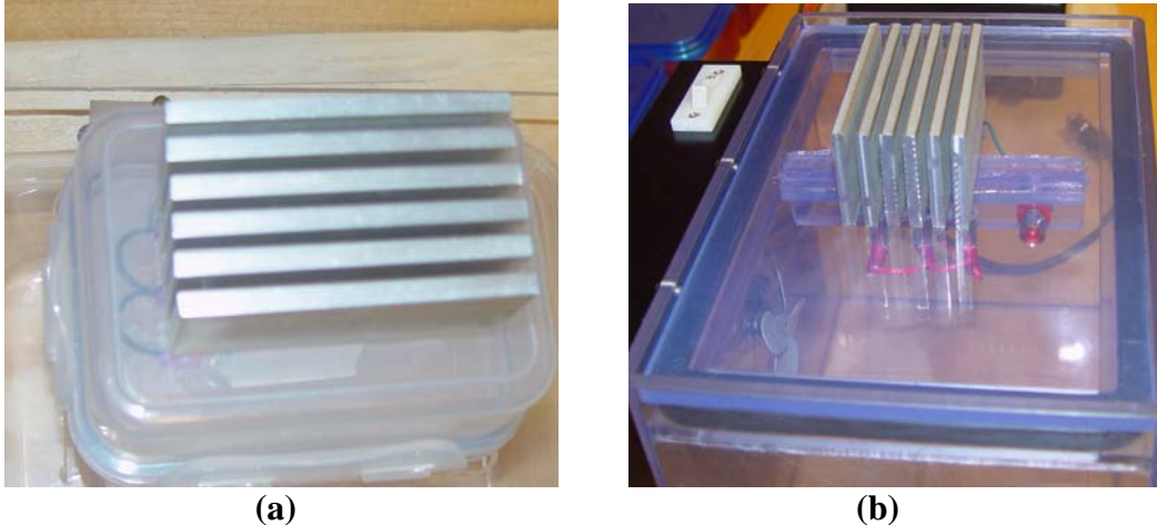
Figure 1. Sensor probes made of (a) aluminum alloy and (b) stainless steel
