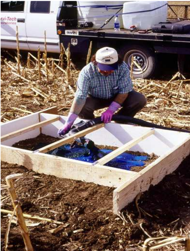
Figure 3. Wooden rectangular frame for flooding the site with dye solution.
