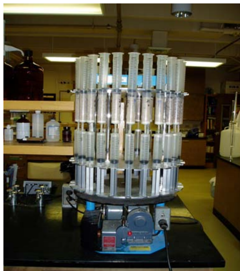
Figure 4. Column experiment setup used to evaluate the cation exchange kinetics between CBNG water and different sizes of St. Cloud zeolites.
