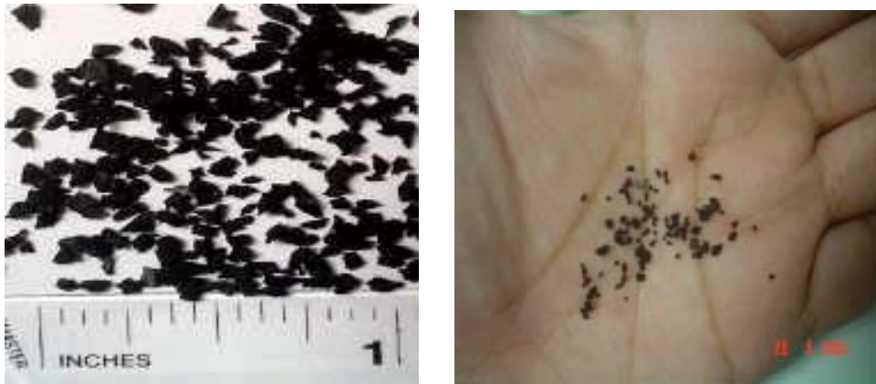
Figure 2 REMA crumb rubber (Mesh 14 – 20). Size of tire rubber particles looks very homogeneous.
