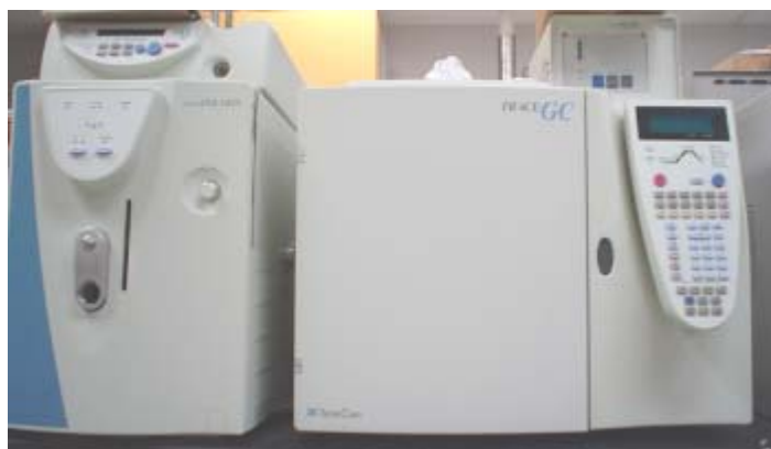
Figure 1. Solid Phase Microextraction set-up (left side) and the Gas Chromatography coupled with Mass Spectrometry Detector (right side)
