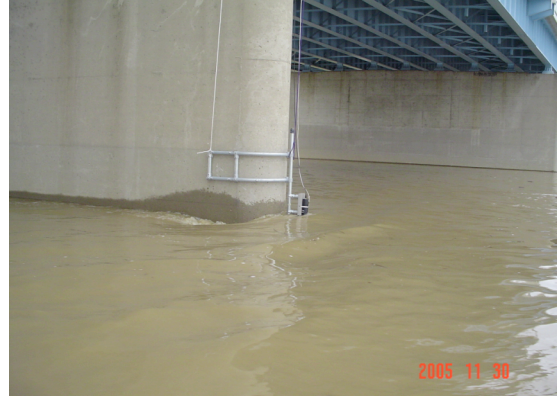
Figure 4. Snapshot of an IMAGENEX deployment at the proposed Hamilton site (ODOT ID-BUT-128-0855). Figure courtesy of Dave Straub (USGS).
