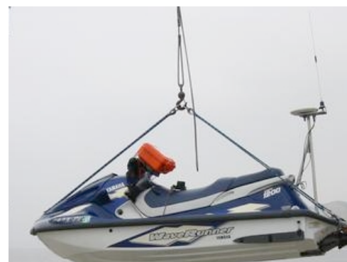
Figure 3. The waverunner survey system is capable of measuring water depths from approximately 0.4 m to 15 m.
