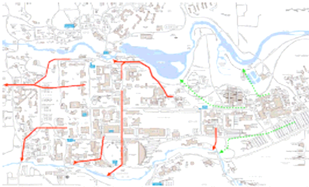
Figure 7. Cornell campus map indicating major storm sewer lines and discharge points. Green, dashed arrows indicate discharge lines where it may be feasible to construct a detention basin or other stormwater management structure.
