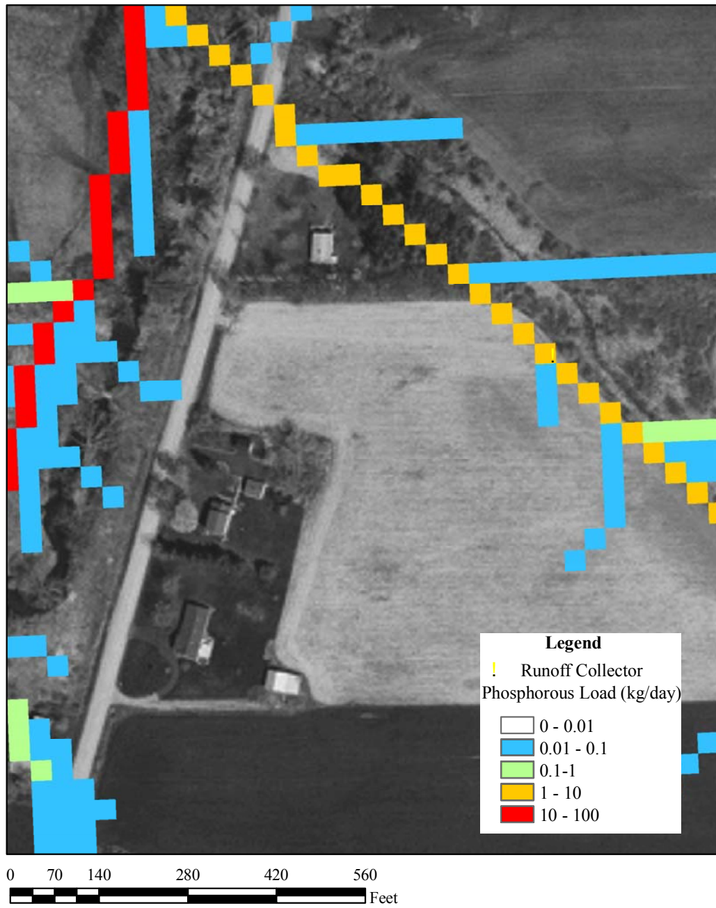
Figure 7 Modeled phosphorous flow paths superimposed on a 2002 aerial photograph of the Clipnock Rd site. The runoff collector for Clipnock Rd is indicated.
