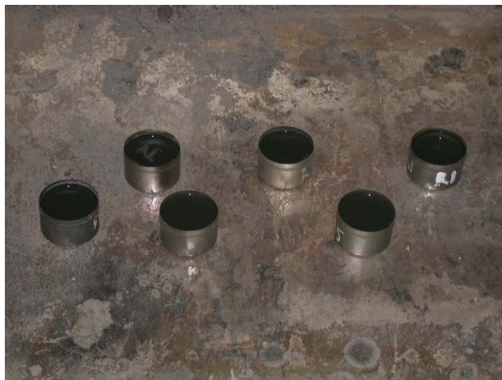
Fig. 3.5 - Laboratory Oven at 110 degrees with soil samples
