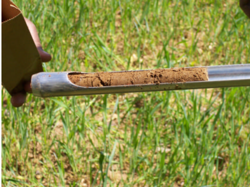
Figure VIII. Soil Sample being examined before sent off to a laboratory for chemical analysis.
