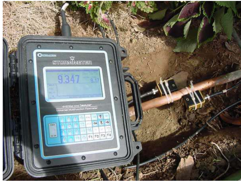
Figure 5.1. Flowmeter and transducers
