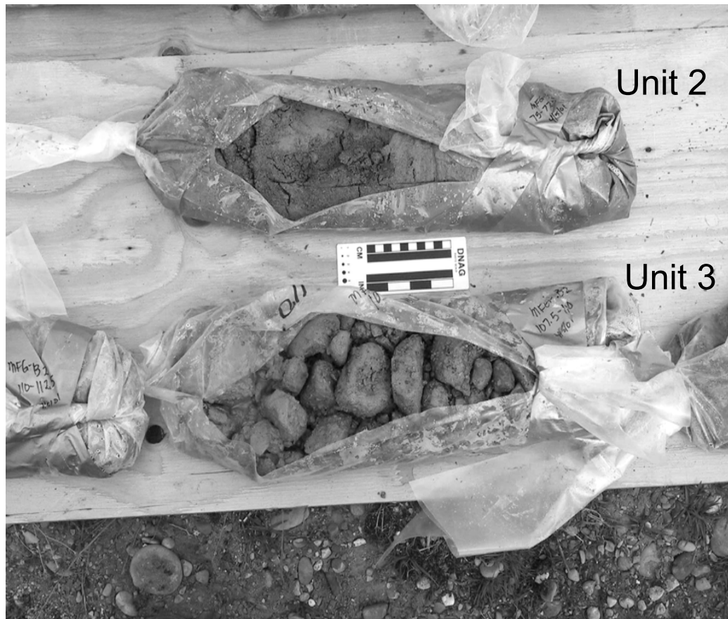
Figure 5. Photograph of core samples showing the fine sand of Unit 2, and the coarse gravels and cobbles of Unit 3. Core came from borehole drilled near the intersection of Russell and Brooks Streets (figure 2). Unit 2 sample is from 75 to 77 feet below land surface. Unit 3 sample is from 107.5 to 110 feet below land surface.
