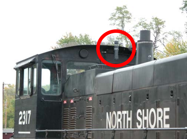
Figure 3. GPS tracking system
