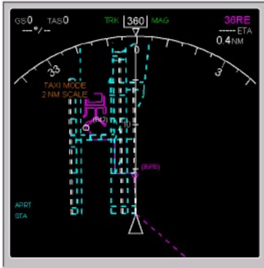
Figure A-13. Smiths Aerospace Flight Management Computer System taxi plan. Photo courtesy of Smiths Aerospace.
