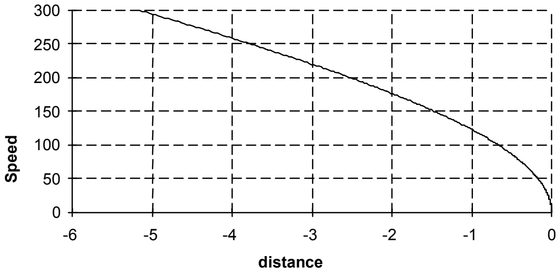
Figure A-5. Full-Service Braking Profile
