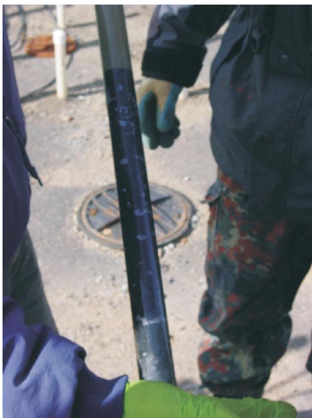
Figure 6. Photograph of a core segment collected from the PRB after 15 months of operation (September 2006).
