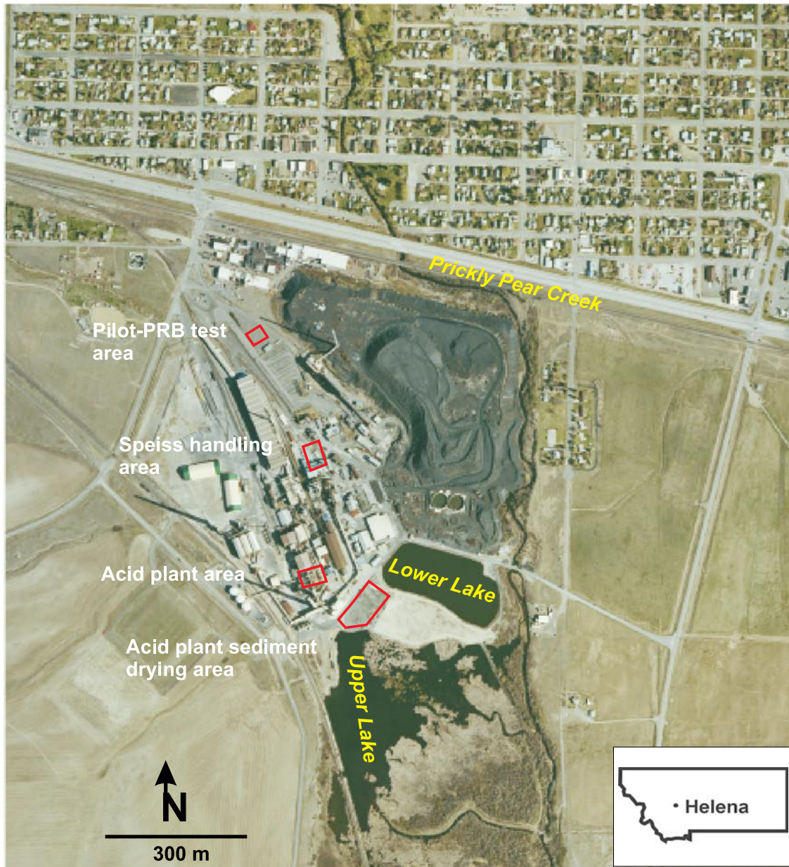
Figure 1. Site aerial photograph showing the ASARCO East Helena smelter, town of East Helena (MT), primary arsenic source zones, and location of the pilot-scale PRB.
