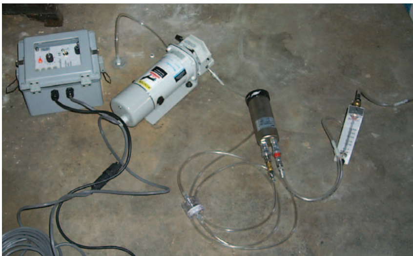
Figure 21. Sample train for sub-slab air collection for radon using scintillation cells.
