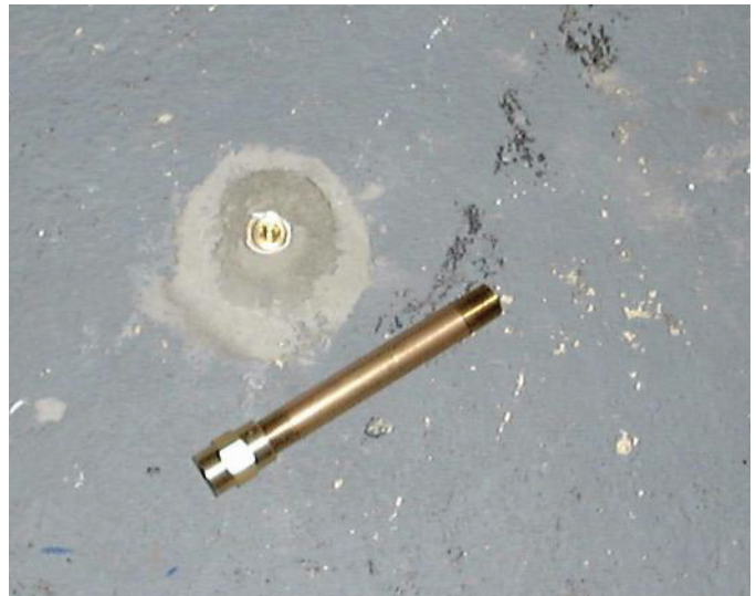
Figure 11. Brass materials used for sub-slab probe construction in homes near the Raymark facility.
