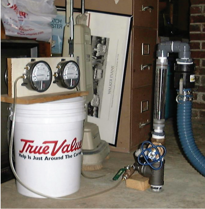
Figure 23. Variable-area flowmeter used for air permeability testing.
