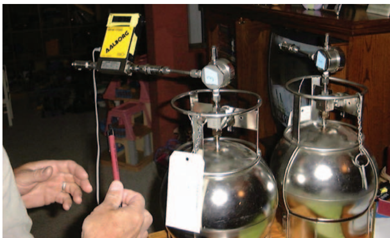
Figure 5. Collection of replicate basement air sample.
