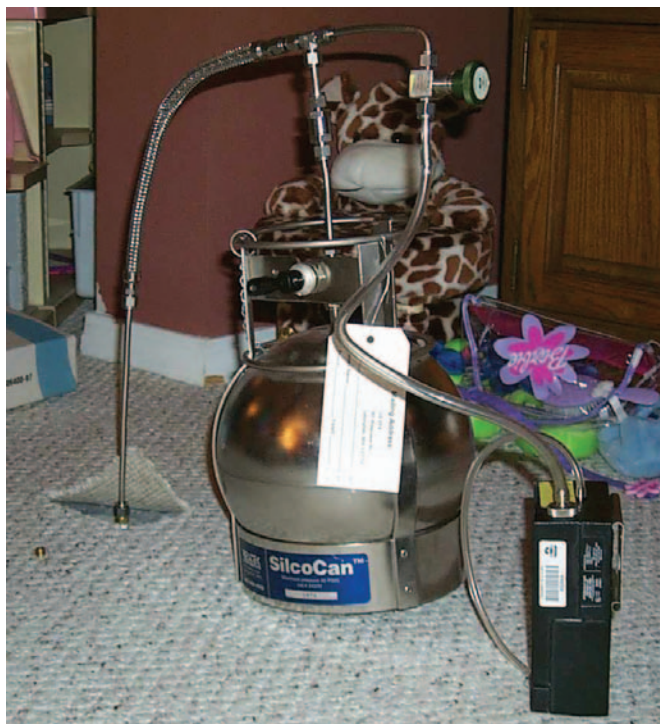
Figure 18. Sample train for sub-slab air collection using EPA Method TO-15.
