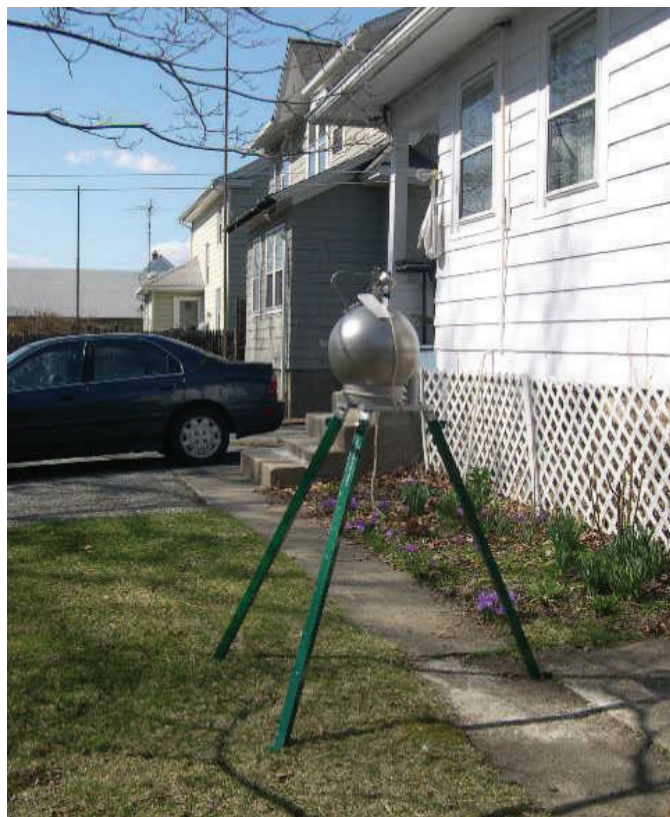
Figure 8. Tripod and six-liter evacuated canister used to collect a 24-hour outdoor air sample during the March 2003 sampling event.
