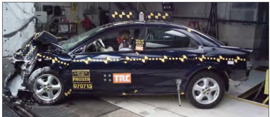
A vehicle-to-deformable-barrier frontal offset test managed by the Volpe Center. (Photo courtesy of Transportation Research Center, East Liberty, Ohio)
