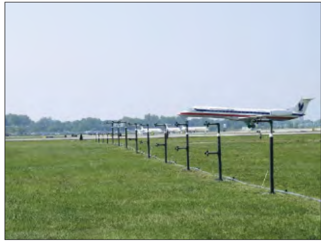
Part of Volpe Center-installed instrumentation for wake measurement at Lambert-St. Louis Airport. Left: Pulsed LIDAR installation. (Photo by Dave Burnham) Right: Windline. (Photo by Kevin Clark)
