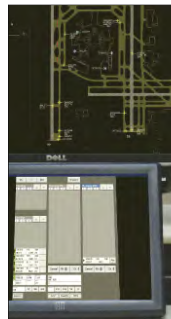
Tower Information Display System: Large flat-panel displays for local and ground controller positions, developed by FAA.
