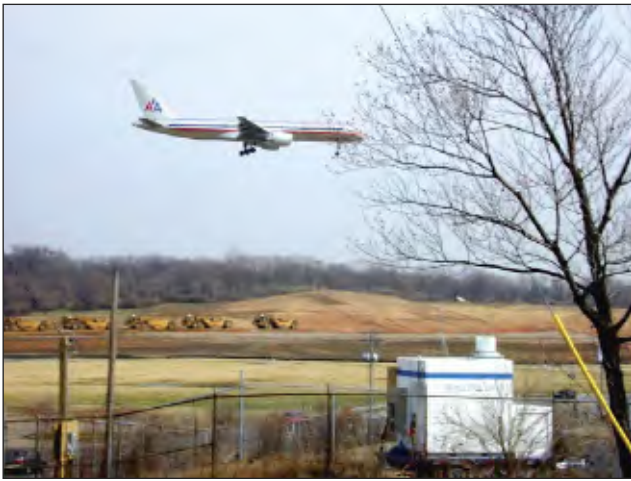
Part of Volpe Center-installed instrumentation for wake measurement at Lambert-St. Louis Airport. Left: Pulsed LIDAR installation. (Photo by Dave Burnham) Right: Windline. (Photo by Kevin Clark)
